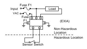
Note: For 120V application, only one fuse is required in the ungrounded circuit of the input line.
